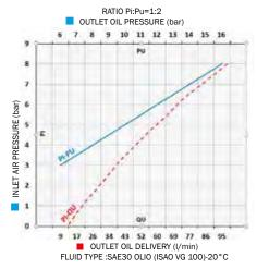
Automatic engine body and shank kit are divided in order to avoid that the fluid enters directly in contact with motor body. These pumps are advised for the transfer of oil and industrial fluids for medium-long distances, guarantee high performance as per delivery capacity (I/min) and also for working pressure.
